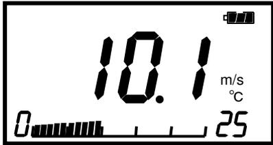
Press **Print** key on the Normal Measurement display (Measurement Mode) to hold the measurement values of the all parameters and print them out. (Air Velocity, Air Temperature and Pressure).
