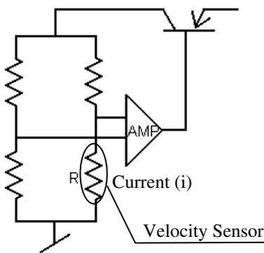
The *Anemomaster* anemometer uses this above mechanism. Generally, a hot-wire anemometer employs a feedback circuit to control the sensor to maintain constant temperature. (Constant Temperature Type)
