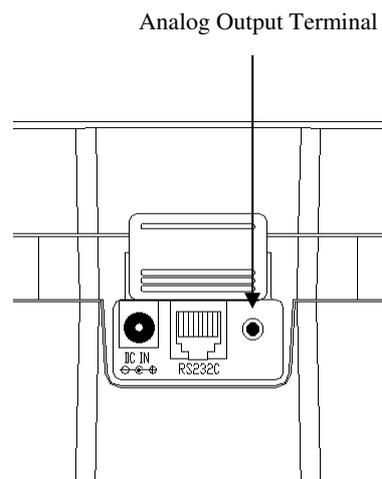
**Output Range:** The output is linear output with the minimum value of 0V and maximum value of 1V.
