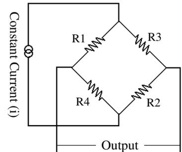
Fig.3 Detection Circuit
