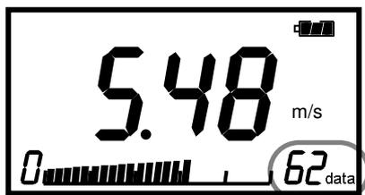
To delete data successively, press **▲** **▼** key to select the data that you want to delete, and press **Clear** key for 4 seconds or longer to delete it. You can delete only one data at a time.
