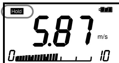
**Hold** mark will appear at the upper right of the display while the reading is held.
