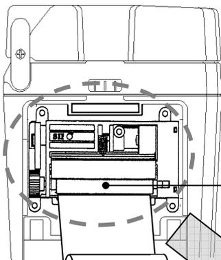
(3) Confirm the sides of the paper - front and back. (As shown in the illustration the inner side of the roll paper shall be facing upwards toward you.) Insert the leading edge of the roll paper underneath the roller.
