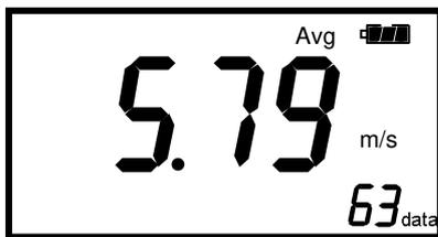
Display the Calculation Mode (by Pressing **Calc.** key in the Normal Measurement screen), and press **Print** key to print out the calculated values (Average, Maximum and Minimum) of all measurement parameters.
