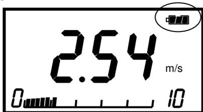
See the Battery Level Indicator in the upper right corner to check the remaining battery level. The battery consumption depends on the air velocity to be measured. When the battery level drops to a level requiring replacement, the indicator starts blinking. Note that it may stop measuring if the indicator starts flashing.
