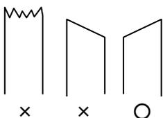
As shown in the left illustration, cut the roll paper diagonally making the right edge is longer than the left. The sensor to detect the roll paper is located at the right side of the roller. Therefore, it would be easier to set the roll paper if the right side of the paper is slightly longer.
