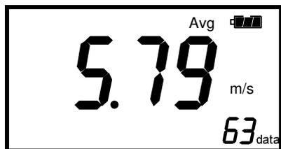
Display the Calculation Mode (by pressing **Calc.** key in the Normal Measurement screen). While holding down **▼** key, press **Print** key to print out the calculation values (Average, Maximum and Minimum) of all the measurement parameters as well as the stored measurement data. Please see the below example of printout.
