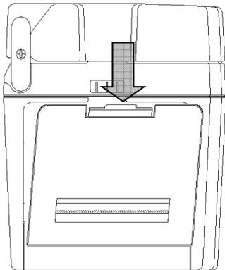
(1) Press lightly where indicated and pull the printer cover to open it.
