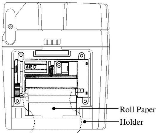
(6) Insert the provided core into the roll paper in order to remove any slack from the roll paper.
