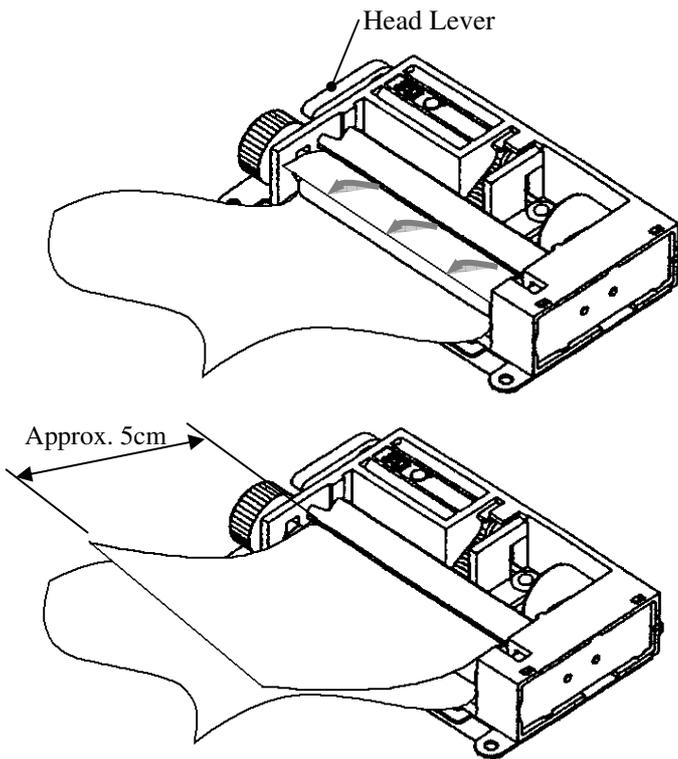
(4) As you insert the leading edge of the roll paper, the roller will automatically rotate to reel in the paper and the paper comes out from the top.
