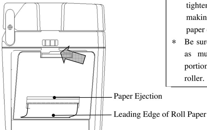
(7) Install the roll paper into the holder as tightening the roll. Close the printer cover making sure that the paper comes out of the paper ejection located on the printer cover.
