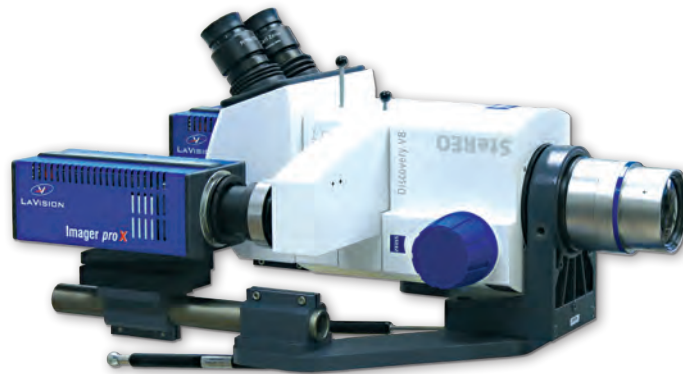
stereoscopic Micro-PIV setup
